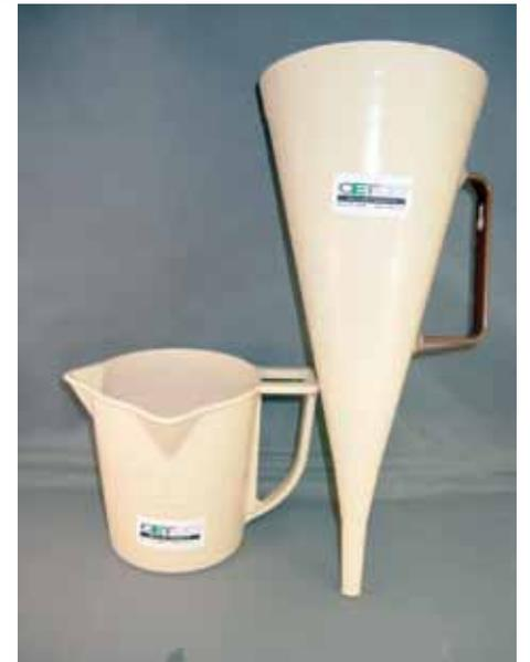
Funnel viscosity reports the thickness of a drilling fluid.
